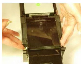
Squeeze nose release buttons, lift
