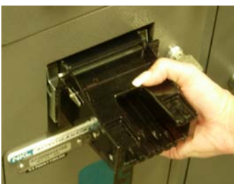
Pull handle under nose to release head assembly
