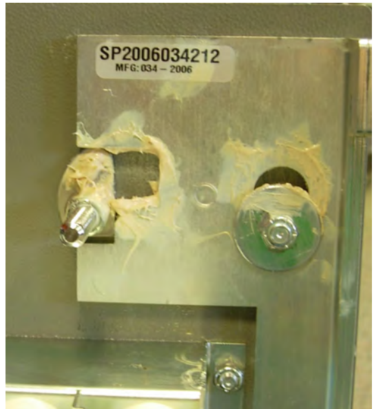
Handle Shaft with Cam (left) and a Guide Bushing (right)
