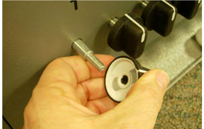
Vend Knobs Slide Off and On
