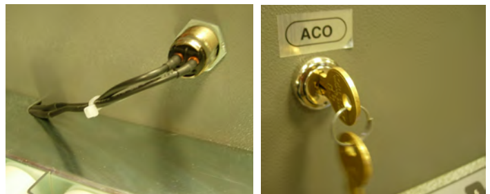
ACO Key Switch from Interior (left) and Exterior (right)
