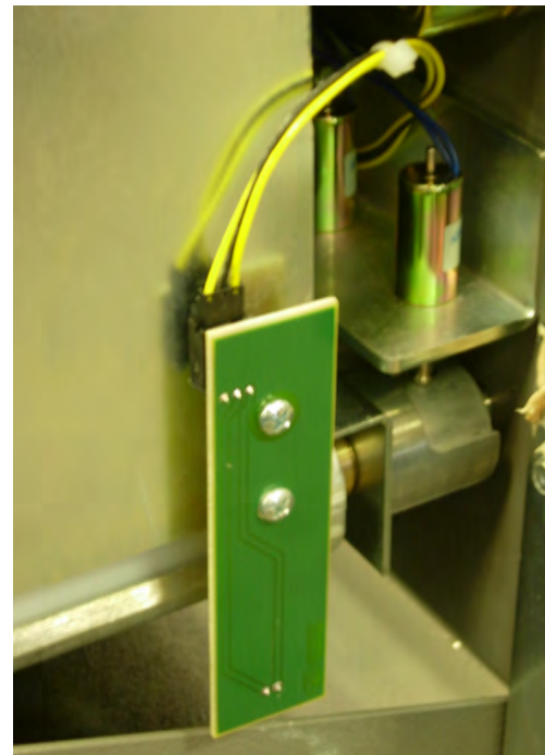
Vend Drop Sensor (Receiver Side Shown)
