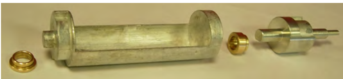
L to R: Rear Bushing, Casting, Front Bushing, Spindle
