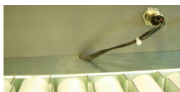
Avoid Pinched Wires (ACO Key Switch Wire)
