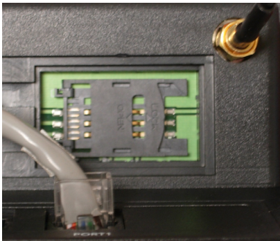
Control Panel SIM Card Port (safe data and antenna cable connections also shown)
