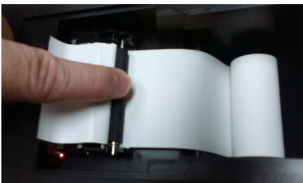
Fig. 7 Roll from beneath, replace roller
